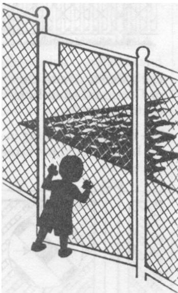
If a gate is properly designed, even if the gate is not completely latched, a young child pushing on the gate in order to enter the pool area will at least close the gate and may actually engage the latch.
